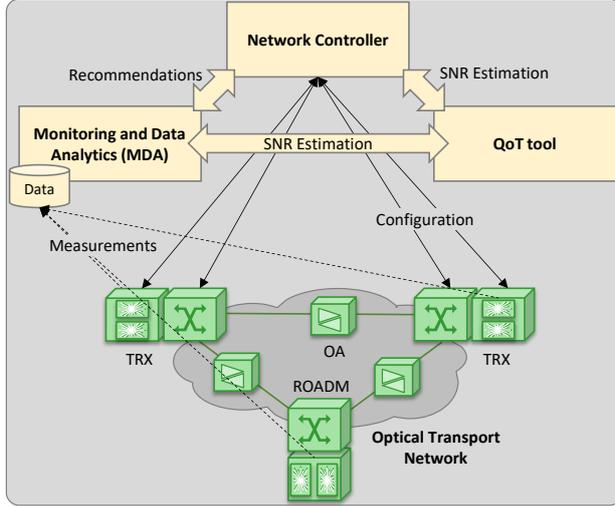
Fig. 1. Overview of the proposed surveillance architecture
