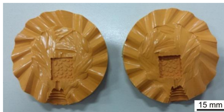
Figure 1. Silicone rubber mold for the metal bezel.
