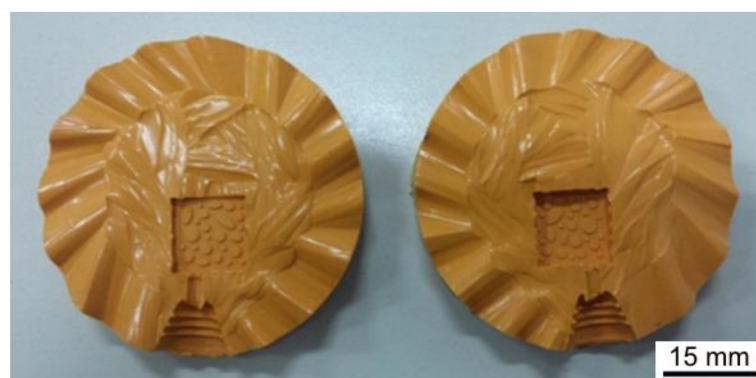
Figure 1. Silicone rubber mold for the metal bezel.
