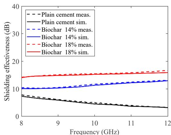
**Figure 7.** Measured and simulated shielding effectiveness values for plain cement, as well as the sample with 14 wt.% biochar and the sample with 18 wt.%. Samples were cured for seven days in water. Measurements were performed after 10 weeks of aging.
