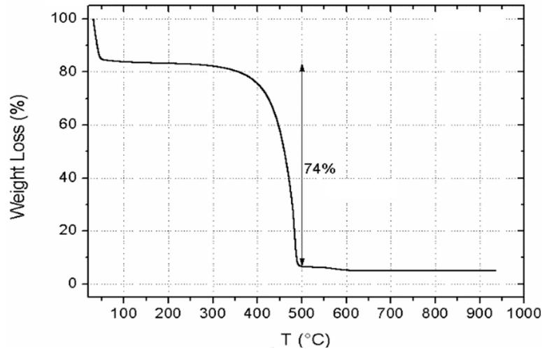
**Figure 5.** Thermogravimetric analysis (TGA) curve of biochar filler.
