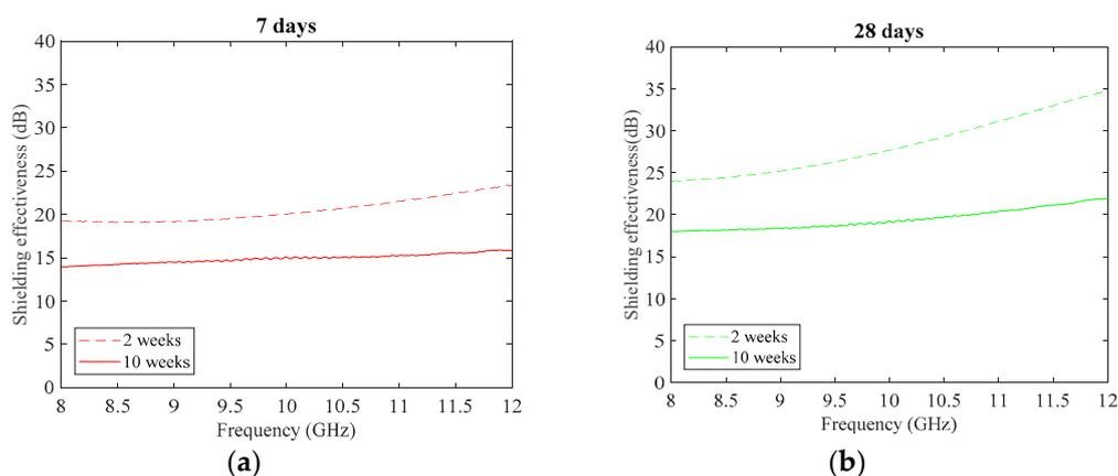
**Figure 8.** Measured shielding effectiveness of cement sample with 18 wt.% biochar: (a) cured in water for seven days; (b) cured in water for 28 days. Measurements were performed after two weeks and 10 weeks.
