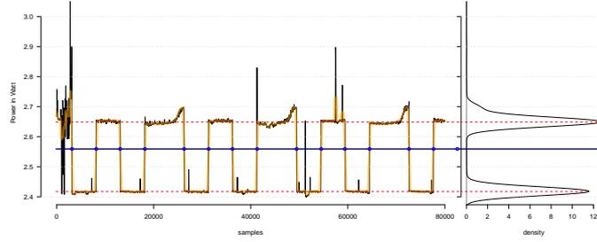
Figure 2: The power signal with embedded markers.
