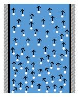
Figure 2.1: Schematic representation of bubbles in the Lagrangian reference frame.
