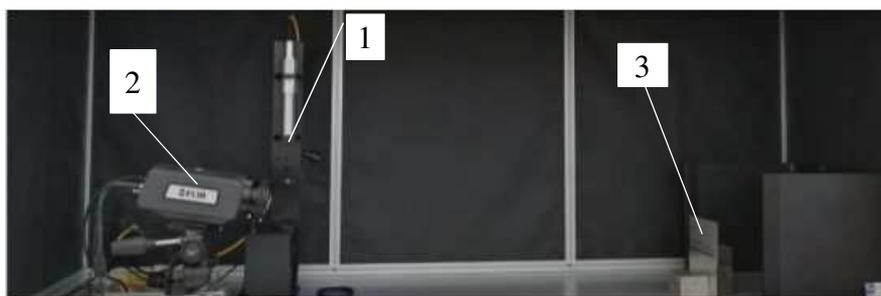
Fig. 1 - Experimental equipment: (1) laser source, (2) IR camera, (3) sample
