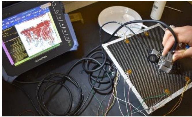
Figure 12: Experimental setup for the C-Scan investigation with Olympus OmniScan SX device.
