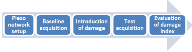
Figure 31: Schematic representation of the experimental procedure.
