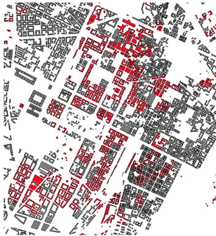
Figure 4-1. Buildings severely damaged (in red) after the earthquake simulation.
