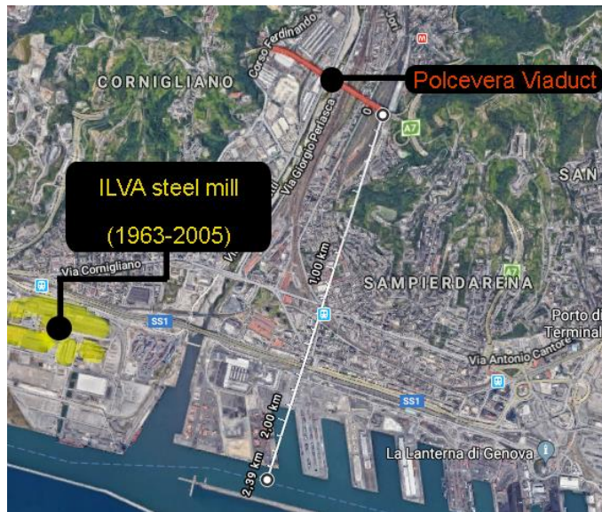
Figure 1: Proximity of the Polcevera viaduct to the main sources of corrosive emissions: the sea and an industrial hub
