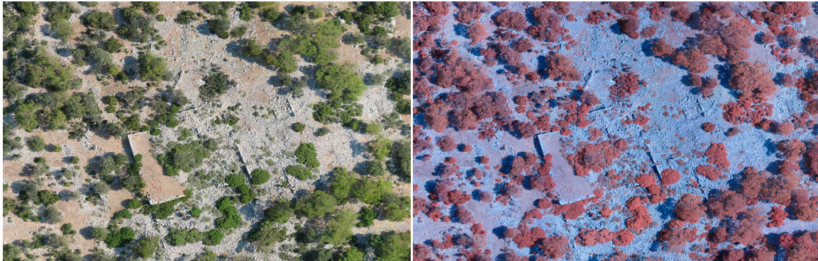
Figure 10. Details from the high-resolution orthomosaics produced for dataset 1 from Metashape Professional: scenario 1—VIS (left), scenario 2—NIR (right).
