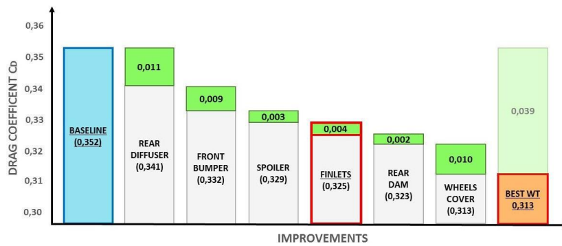
Fig. 8. Wind Tunnel best results at 70 km/h
