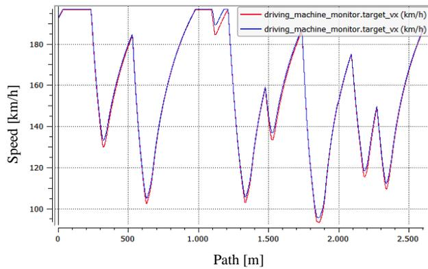
Figure 193 – Speed profile (red: base, blue: controlled)
