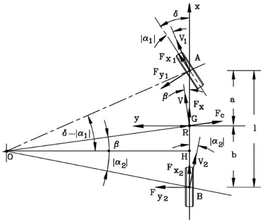
Figure 2 - Monotrack model [15]
