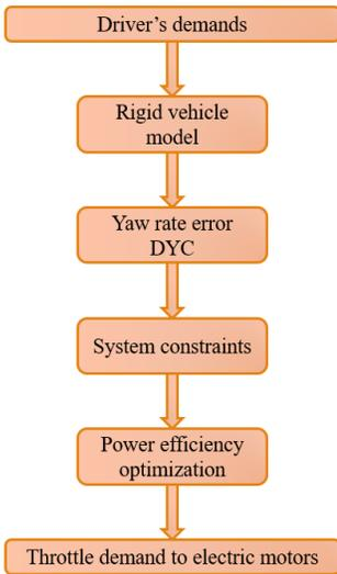
Figure 7 – Conceptual block scheme of the control model
