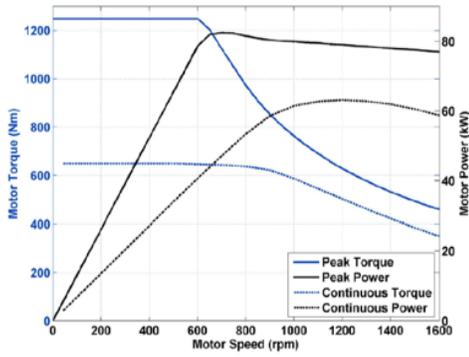
Figure 8 – Torque and Power vs. Speed [25]
