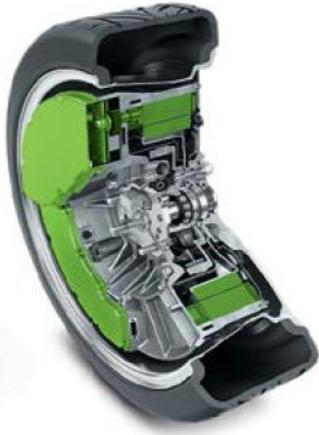
Figure 1 - Schaeffler's E-Wheel drive [11]
