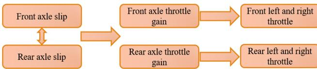
Figure 6 – Traction control for slip reduction working method
