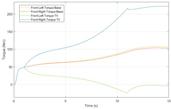
Figure 11 – Front left and front right wheel torques
