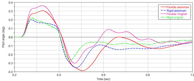
Fig. 8. Pitch angle evolution - Pothole encountering
