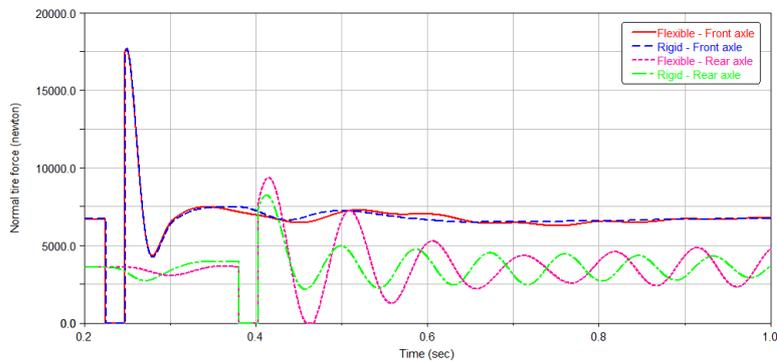
**Fig. 6.** Original configuration: tire normal forces - Pothole encountering
