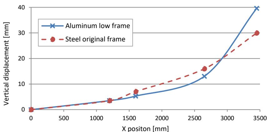
**Fig. 2.** FEM frame torsion simulation results
