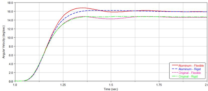
**Fig. 5.** Yaw rate evolution - Step steering
