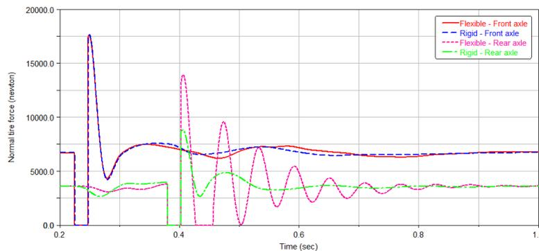
**Fig. 7.** Aluminum frame: tire normal forces - Pothole encountering
