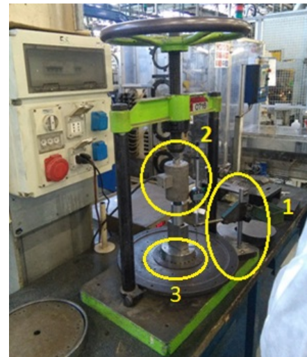
Figure 8. Press bench for drive plate axial compliance characterization.
