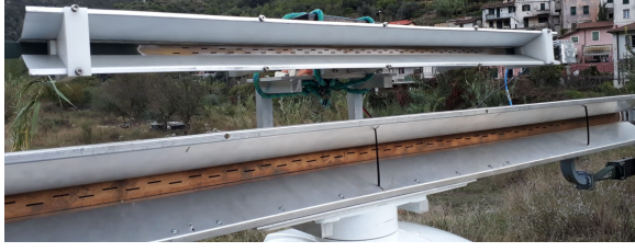
Fig. 5. Detailed view of the TX and RX antennas.
