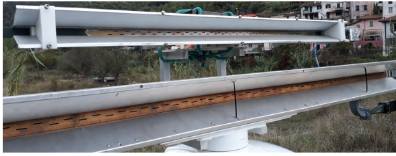
Fig. 5. Detailed view of the TX and RX antennas.
