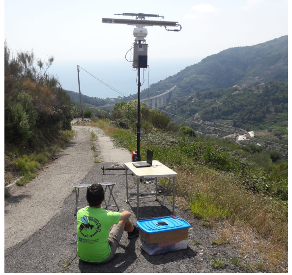
Fig. 2. Standard radar setup. The TX and RX antennas are visible on top of the system, while the 4U case rack is hanging right below the rotary joint. A telescopic tower helps to operate the radar up to about 6 meters from the soil in order to avoid obstacles, such as trees or bushes.
