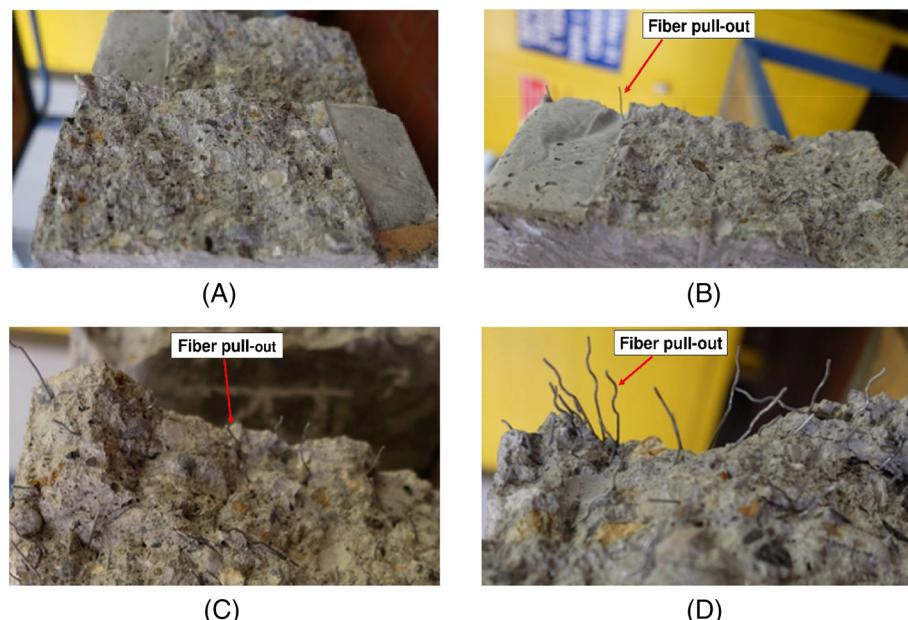
**FIGURE 10** Fracture surfaces. A, FRC-20-04; B, FRC-20-15; C, FRC-20-75; D, FRC-20-100
