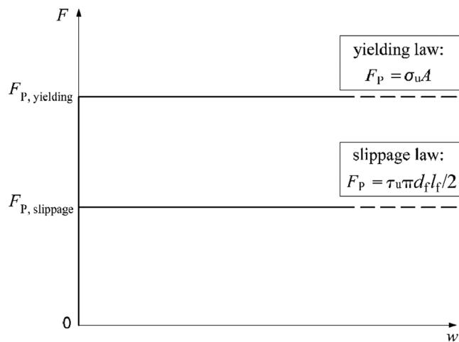
**FIGURE 2** Reinforcement constitutive laws: Fibre yielding or slippage
