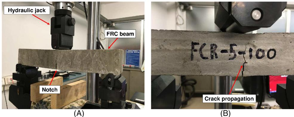
**FIGURE 7** A, Experimental set-up; B, Crack propagation process
