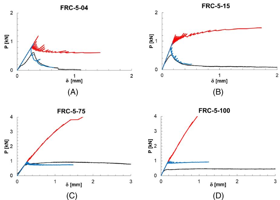
**FIGURE 11** Experimental results vs numerical model for the specimen with  $h = 5$  cm. A, FRC-5-04; B, FRC-5-15; C, FRC-5-75; D, FRC-5-100. The red and blue curves are obtained by the numerical model, in the case of yielding and slippage mechanism respectively. The black curve indicates the experimental results
