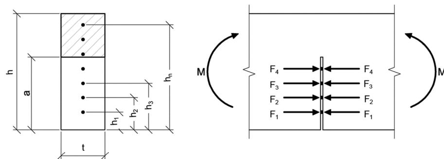
**FIGURE 1** Fibre-reinforced brittle-matrix beam model
