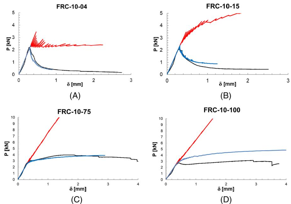
**FIGURE 12** Experimental results vs numerical model for the specimen with  $h = 10$  cm. A, FRC-10-04; B, FRC-10-15; C, FRC-10-75; D, FRC-10-100. The red and blue curves are obtained by the numerical model, in the case of yielding and slippage mechanism respectively. The black curve indicates the experimental results
