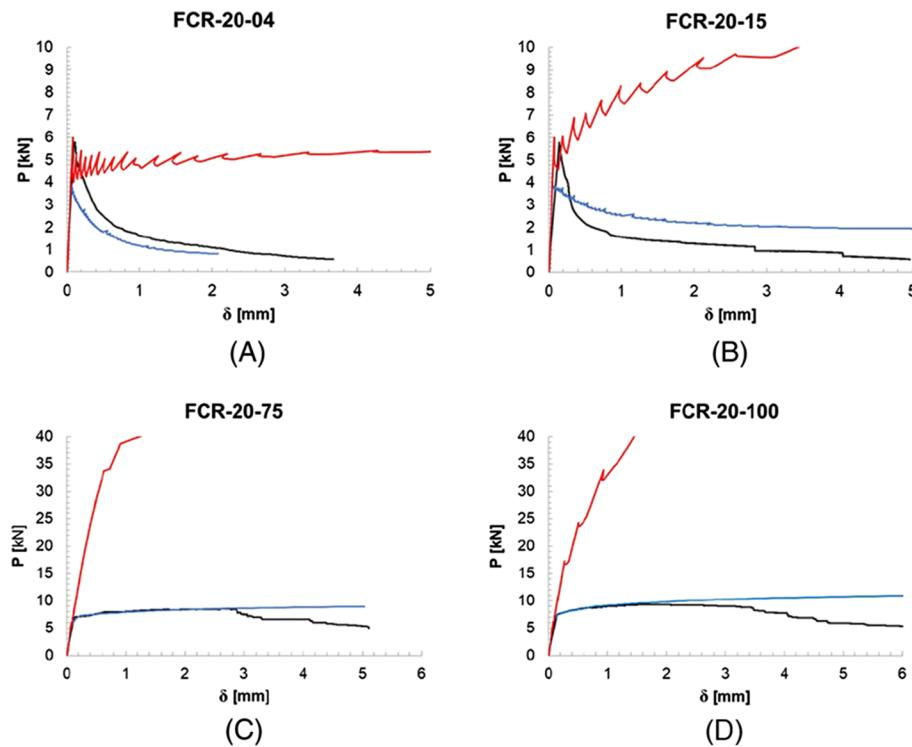
**FIGURE 13** Experimental results vs numerical model for the specimen with  $h = 20$  cm. A, FRC-20-04; B, FRC-20-15; C, FRC-20-75; D, FRC-20-100. The red and blue curves are obtained by the numerical model, in the case of yielding and slippage mechanism respectively. The black curve indicates the experimental results
