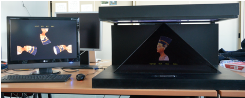
Figure 9: Overall setup of the system used for demonstrating the virtual exhibition of the bust of Queen Nefertiti.
