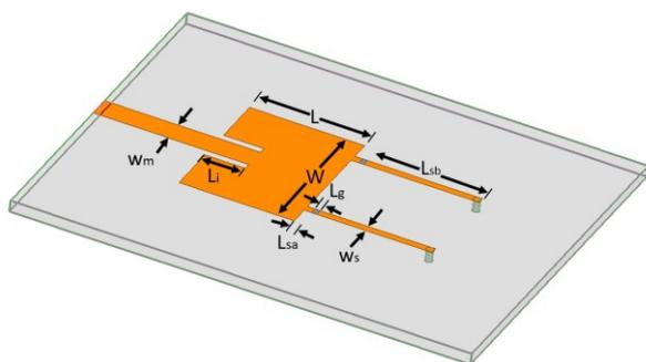
**Fig. 1** Geometry of the reconfigurable graphene antenna.
