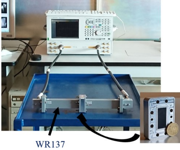
Fig. 4 Waveguide measurements with VNA. See the waveguide spacer in the inset
