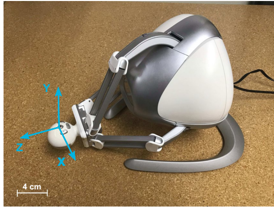
Figure 1. The Novint Falcon game controller with overlaid global coordinate system, describing the end-effector's motion in three dimensions.
