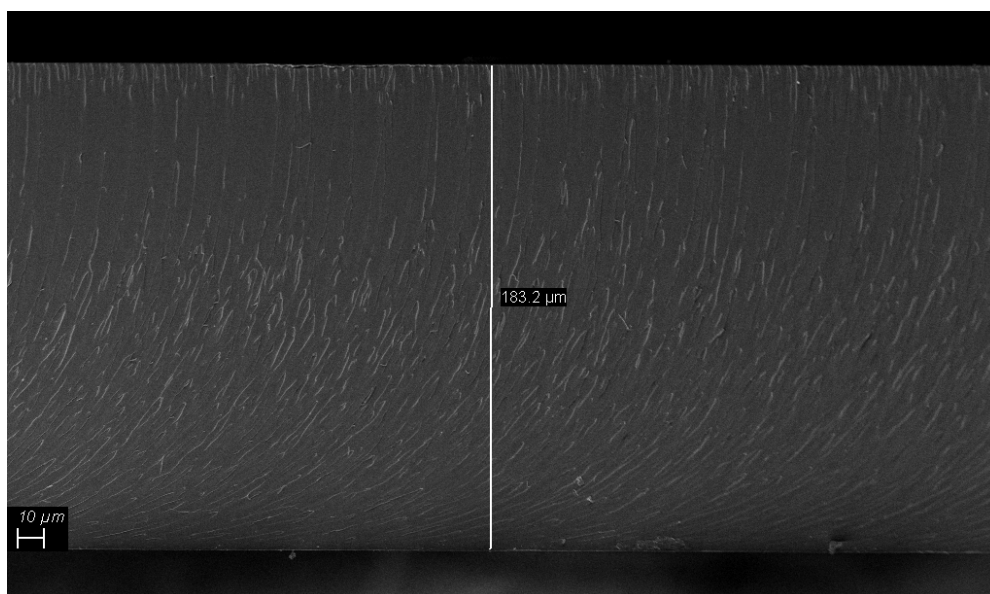
Figure 3. FESEM capture of unfilled UV-LED cured EB150 film on the transversal plane.
