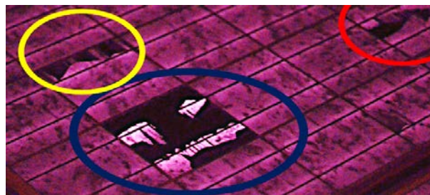
Fig. 11. EL detail of defective cells in the modules of Fig. 9.
