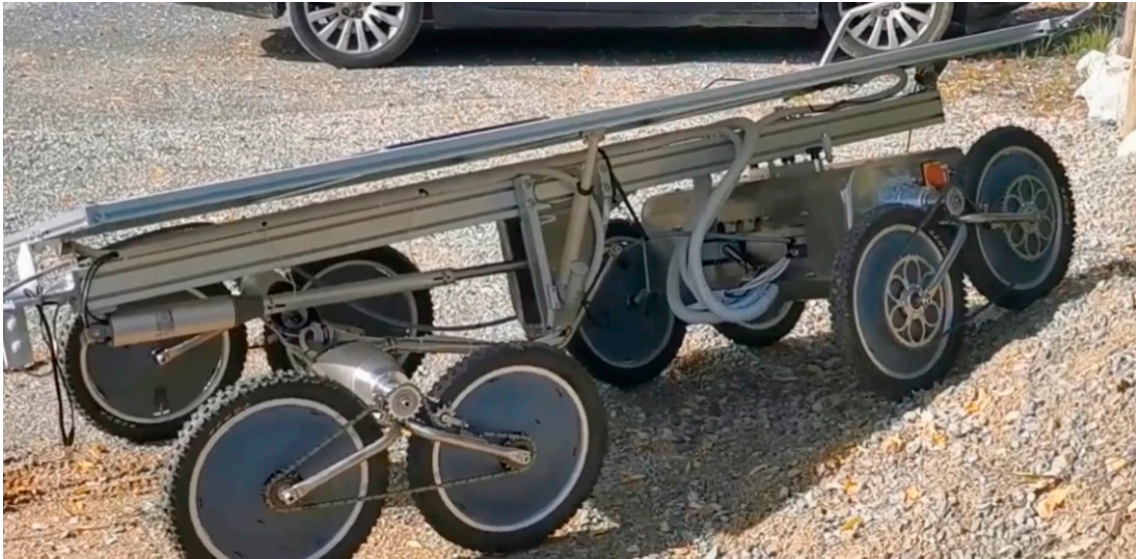
Figure 13. Agri.q02 can modify its configuration during the motion to adapt to irregular terrains.
