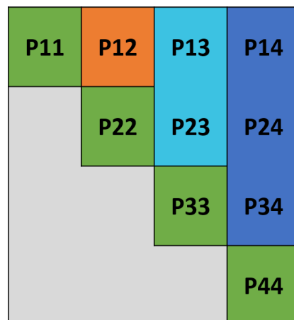
Figure 5. Block-streaming method with 4 blocks ( B/B_{max} = 4 ).
