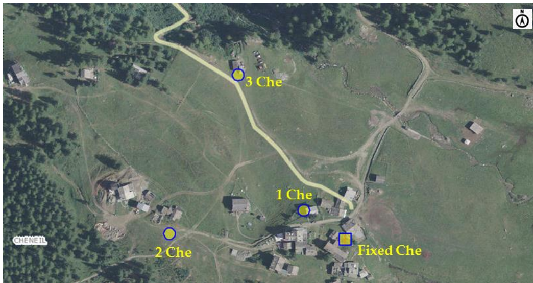
Figure 6. Acoustic measurement points in the Cheneil valley: one for fixed monitoring (square) and the others for short-term monitoring (circles). Source: http://geonavsct.partout.it/pub/GeoCartoSCT/index.html .
