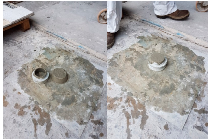
Figure 8. Spreading test results. No loss of shape is shown.
