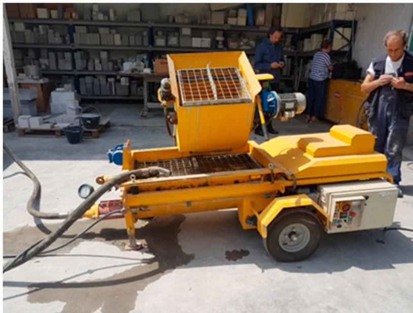
Figure 4. S8 EVM machinery creation of TEK.SP.ED s.r.l. used for eco-mortar for plaster mix design.
