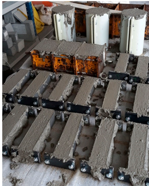
Figure 7. Plaster specimens prepared for physical-mechanical tests, according to standard UNI EN 998-1 and 2.
