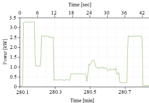
Figure 4. (2.3) Printing phase: data acquisition and identification of the main layer subphases.
