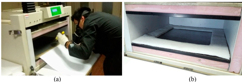
Figure 3. (a) Coating of the lower Heat Flux Meter (HFM) plate; (b) Polyester ring.
