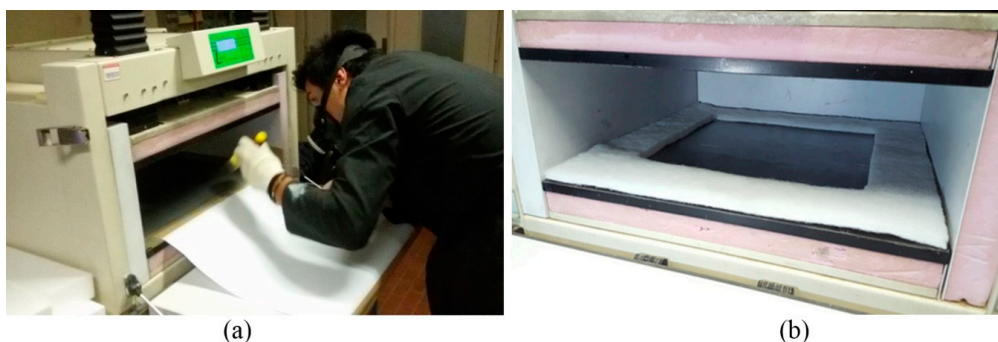
Figure 3. (a) Coating of the lower Heat Flux Meter (HFM) plate; (b) Polyester ring.
