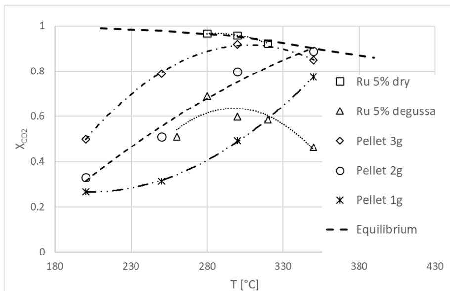
**Figure 1** CO<sub>2</sub> conversion in function of temperature for all runs
