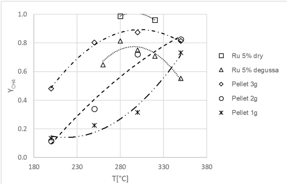
**Figure 2** CH<sub>4</sub> yield in function of temperature for all runs
