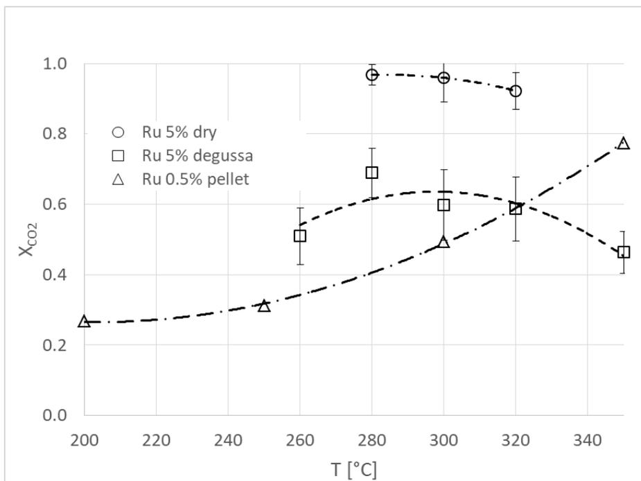
**Figure 3** CO<sub>2</sub> conversion at GHSV = 2 Lh<sup>-1</sup>g<sup>-1</sup> for the three catalysts
