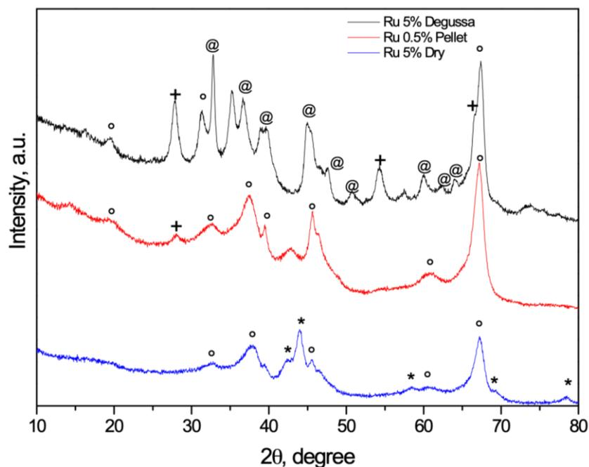
**Figure 4** Powders XRD patterns of the commercial catalysts
