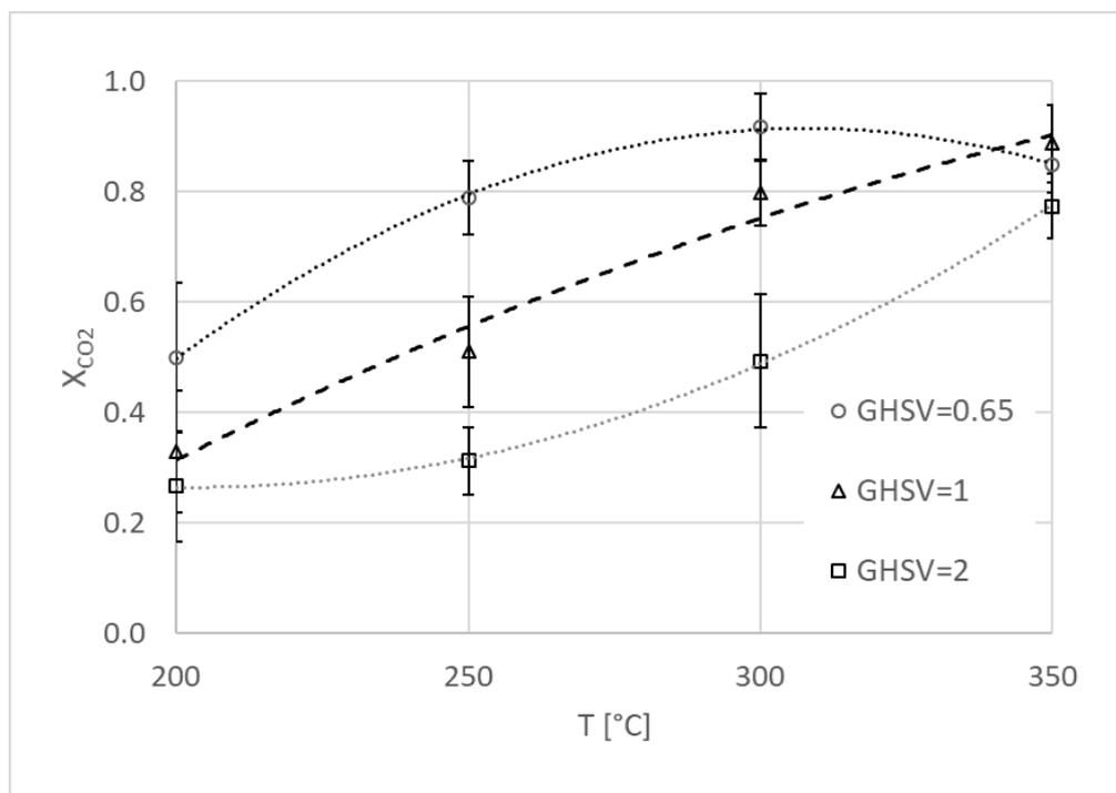
**Figure 6** CO<sub>2</sub> Effect of reaction temperature and GHSV on X<sub>CO2</sub> conversion using pellets Ru 0.5%.
