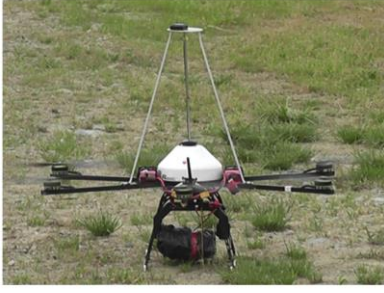
Fig. 4 UAV equipped with on-board GNSS-R sensor
