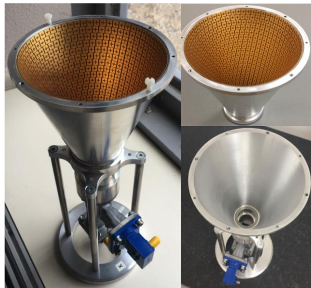
Fig. 10. Final Metahorn Engineering Model.
