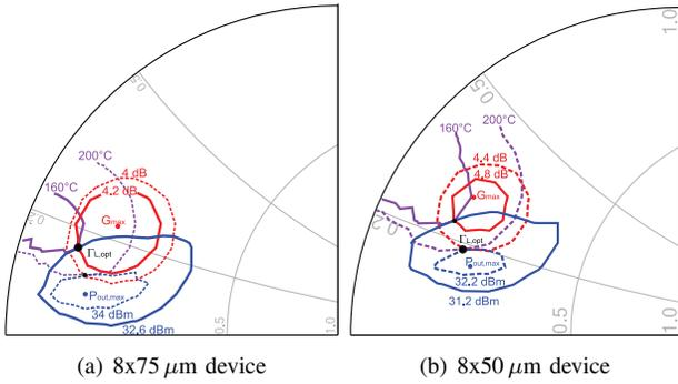
Fig. 6. Load-pull results at  $V_{DS} = 11.25$  V, 1 dB compression.
