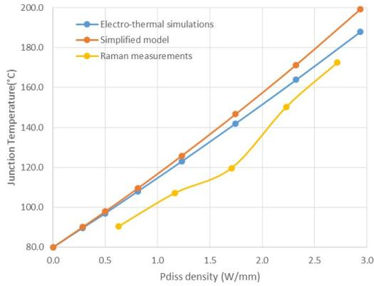
Fig. 4. Junction temperature as a function of dissipated power density: comparison between electro-thermal simulations, simplified model predictions and Raman measurement results ( $8 \times 50 \mu\text{m}$  device).
