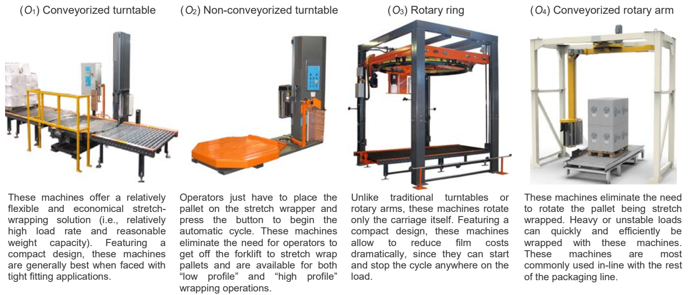
Fig. 3. Schematic representation and short description of four design concepts of automatic stretch-wrapping machines.
