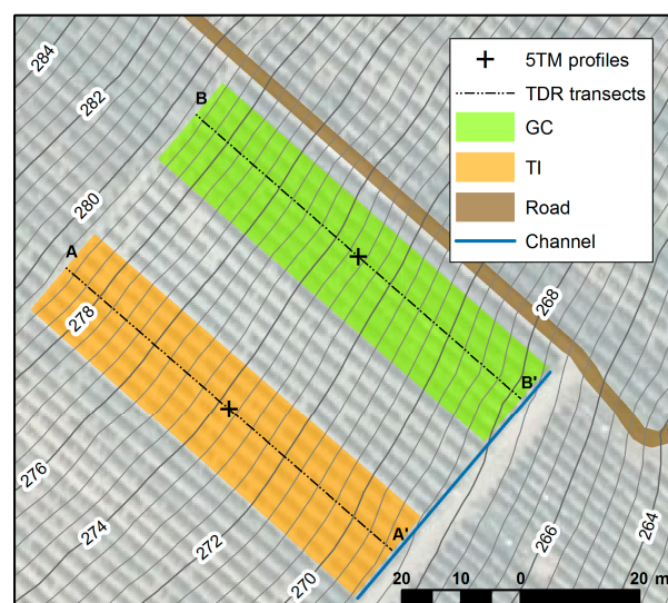
Figure 6. Carpeneto site. Plot of the experimental field. Grass Cover (GC) and Conventional Tillage (TI) represent the two investigated cultivation techniques. The two dotted lines A–A’ and B–B’ represent the investigated TDR transects.
