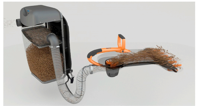
Fig. 11. Backpack combine harvester functioning.
