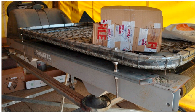
Fig. 5. Self-produced chestnut deburring machine.
