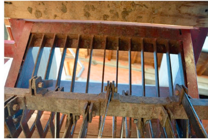
Fig. 5. Self-produced chestnut deburring machine.
