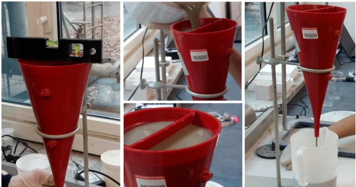
Figure 2. Flowability test device installed in laboratory. The filling of the Marsh cone and the measurements of the flow time phase are shown in the center and on the right respectively.
