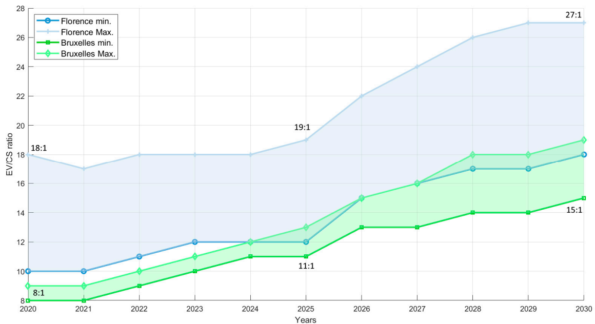
Figure 11. Publicly accessible charging infrastructure electric vehicle (EV)/CS ratio for Florence (light blue) and Bruxelles (light green).
