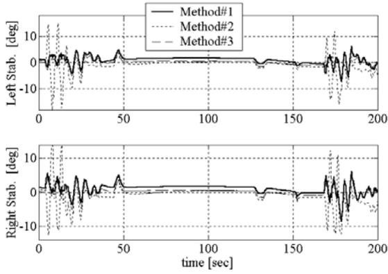
**Figure 10.** Left/Right Stabilator deflections (*Man #1* = no failure)
