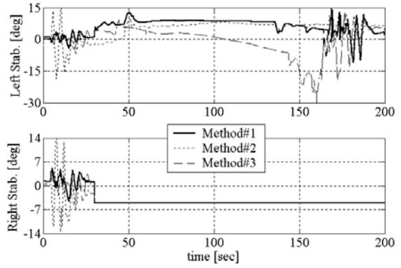
**Figure 11.** Left/Right Stabilator deflections (*Man #2* = stabilator failure)
