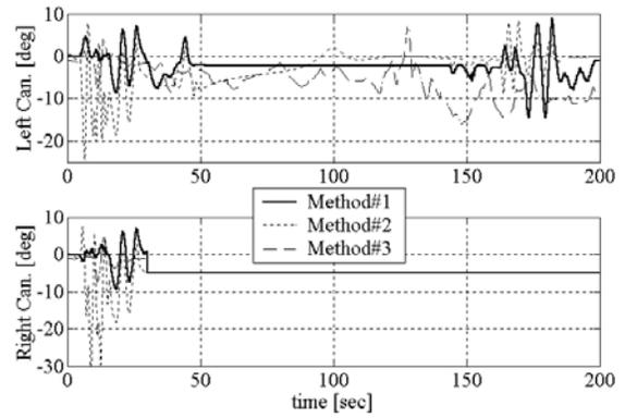
**Figure 13.** Left/Right Canard deflections (*Man #3* = canard failure)
