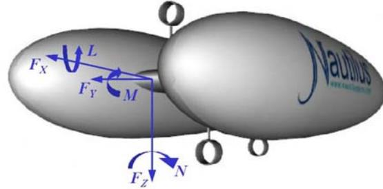
Figure 3. Force and moments acting on the airship
