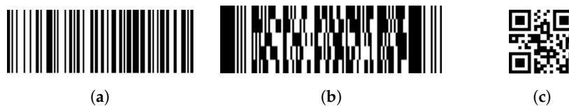
Figure 1. Barcode technology evolution: (a) code 128, (b) code PDF417 and (c) quick response (QR) code.
