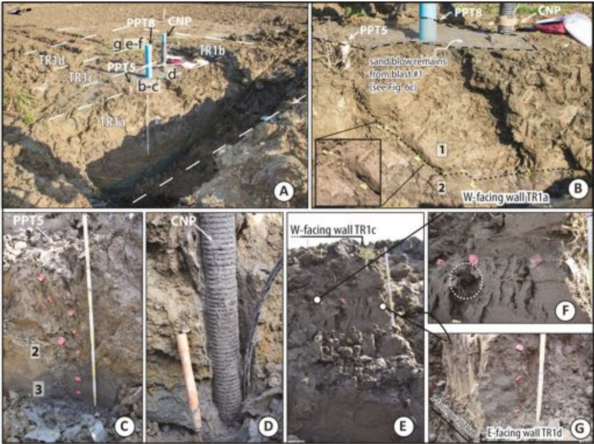
650 Fig. 13. Geometrical arrangement of the trenches (a); details of the most significant features 651 exposed in the walls. Sand boils from the blast test (b) were generated by sand moving upward 652 using the PPT5 pore pressure transducer, colored flags in (c), and the external part of the CNP 653 profilometer (d) as conduits. Sand from CNP moved sub-horizontally, as shown by yellow flags, in 654 (b). The white dashed circle in (f) indicates the remnants of the vegetation at the ground surface, 655 covered by the 2012 sand blow (bottom of the blow marked by colored flags in e, f). Details of the 656 2012 vertical path (colored flags) developed along a thin fracture in (g).
