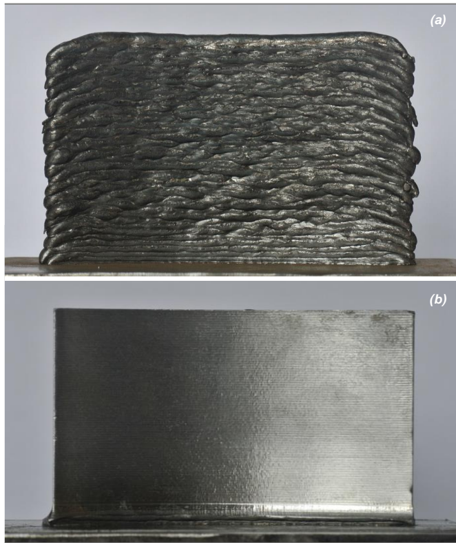
Fig. 4 Detail of (a) as-deposited and (b) machined airfoil.
