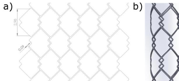
Figure 4 a) 2D mesh and b) 3D model of a stent to be produced by SLM in the target vessel diameter (build direction is vertical to the image plane and parallel to the axial direction of the stents).
