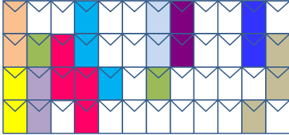
Fig. 8: Example of clustering result. Roof 1, m \times n = 8 \times 6 , \epsilon = 4\% , reconfigurable elements = 34 (i.e. 70%).
