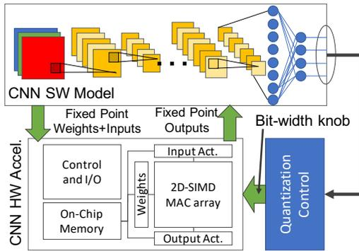
**Figure 4: Proposed dynamic bit-width reconfiguration method for CNNs.**
