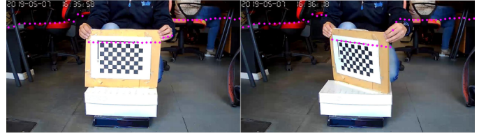
Fig. 3. Laser points projected in the image plane.
