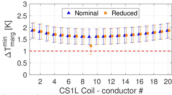
Fig. 15.  $\Delta T_{\text{marg}}^{\text{min}}$  in CS1L module with nominal (blue triangles) and reduced (orange squares)  $\dot{m}$  in most critical channel (#9) for a virgin conductor. The horizontal red line shows the minimum temperature margin requirement for a virgin conductor.
