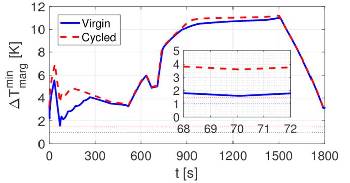
Fig. 13. Evolution of the absolute  $\Delta T_{\text{marg}}^{\text{min}}$  in the CS with the  $n\tau$  evaluated for the virgin (solid blue) and cycled (dashed red) conductor. The minimum requirements are also reported as horizontal dotted lines.
